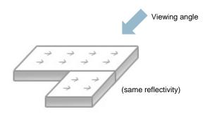
The variation of the particulate distribution pattern between two separate pieces seamed together may be obvious and easy to notice if not fabricated as suggested in this technical bulletin, On your Pearl particulates project we strongly suggest that you experiment, prior to actual fabrication, with the methods and procedures described above.
